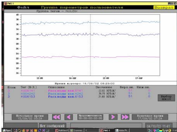
Fig. A - Monitoring of defective flowmeters before Unit 3 shutdown on 16.09.02, The lines show instabilities in the operation of the flowmeters.
